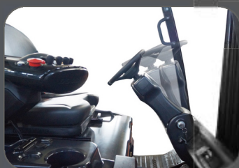
Fully Adjustable Steering Column
